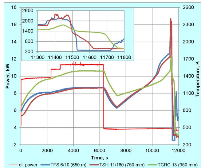
Fig. 2. QUENCH-16 test conduct.
