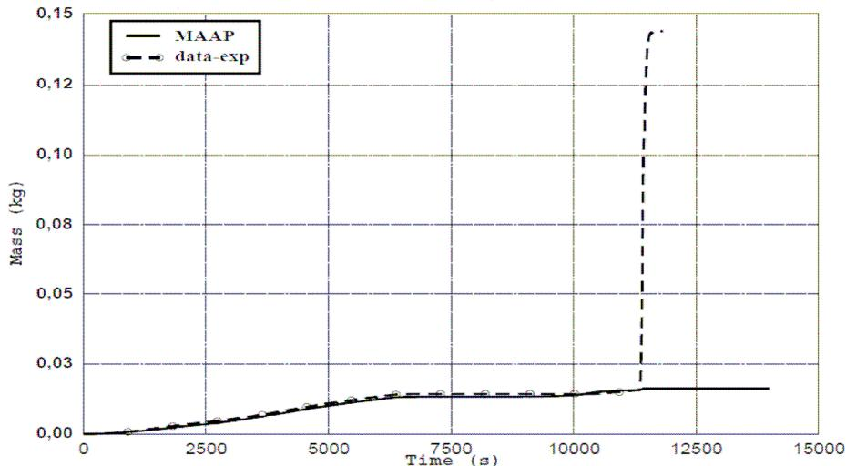
Fig. 7: Hydrogen production for the experiment (in dashed lines) and for the simulation (in solid lines)
