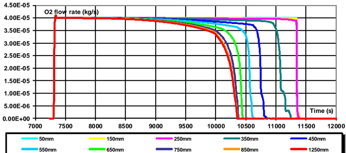
Fig. 8: Calculated oxygen flow rates during the air phase
