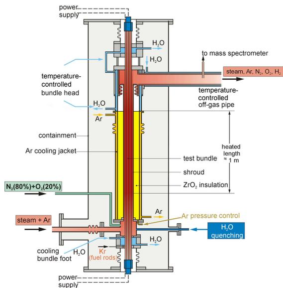
Fig. 1. Containment and test section.
