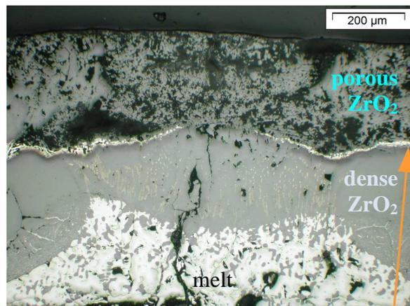
Fig. 4. Cladding structure elevation 550 mm: nitrides between inner dense and outer porous oxide layers
