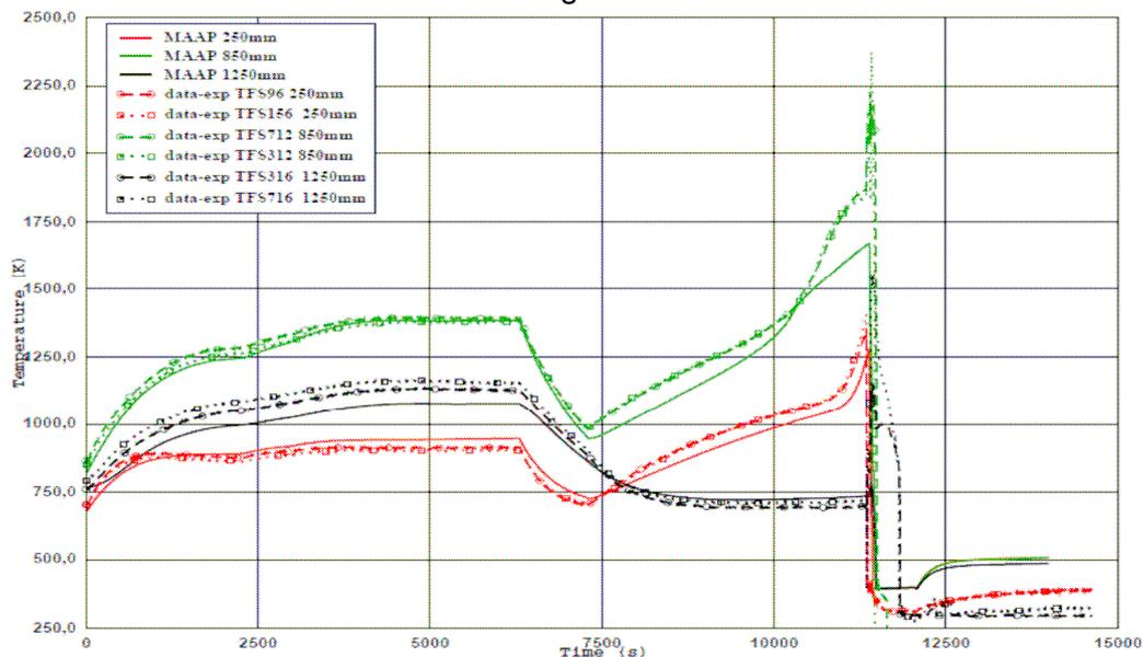
Fig. 6. Temperatures evolution of the bundle for the experiment (in dashed lines) and for the simulation (in solid lines) at 250mm, 850mm and 1250mm of height (in red, green and black,
