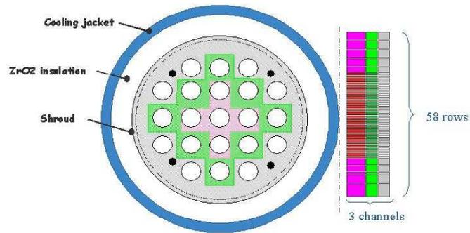
Fig. 5. Mesh of QUENCH-16 experiment in MAAP4
