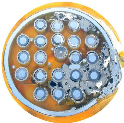
Fig. 3. Bundle cross section at 430 mm: frozen melt relocated from upper elevations
