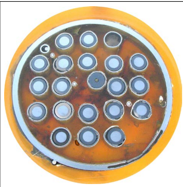
Figure 8. Bundle cross section at 830 mm: minor melting of some cladding segments
