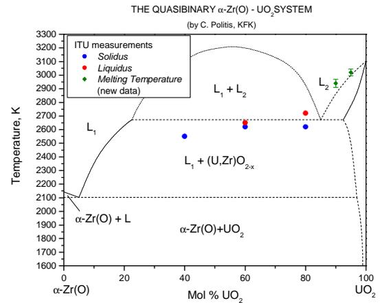
**Figure 13:  $\alpha$ Zr(O)-UO<sub>2</sub> pseudo-binary diagram, with ITU experimental results**
