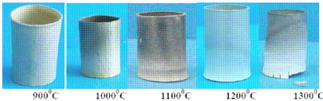
Figure 4: CANDU-type Zry-4 after oxidation in humid atmosphere at INR
