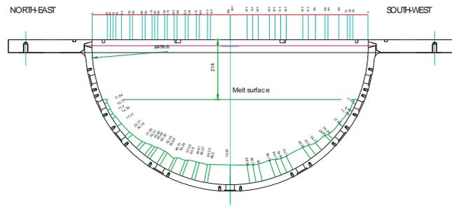
Figure 5: Crust thickness after LIVE L-1 test
