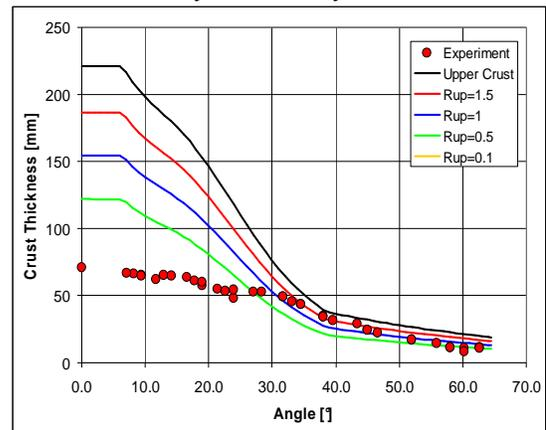
Figure 6: Comparison with experiment of LIVE L1 crust thickness estimated with the ACOPO correlation and various boundary conditions at the pool upper surface.
