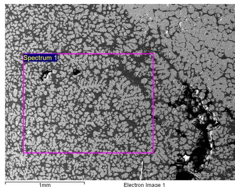
**Figure 14: SEM Micrograph of a VULCANO VB-U6 sample performed by ITU within the round robin near the boundary between a corium-rich (right) and a concrete-rich (left) liquid.**
