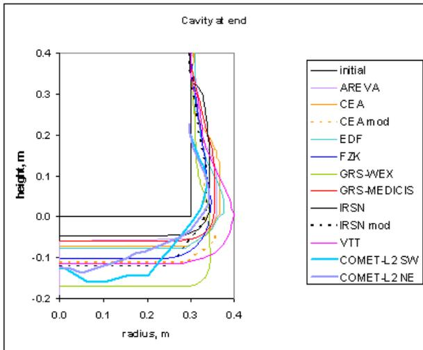
Figure 11: Benchmarking of computed COMET L2 final ablation profiles
