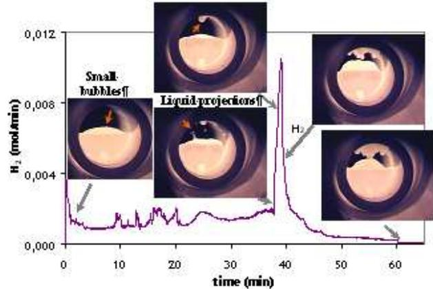
**Figure 3: Phenomena observed in BECARRE during the oxidation of a steel - 5%B<sub>4</sub>C mixture at 1289°C**
