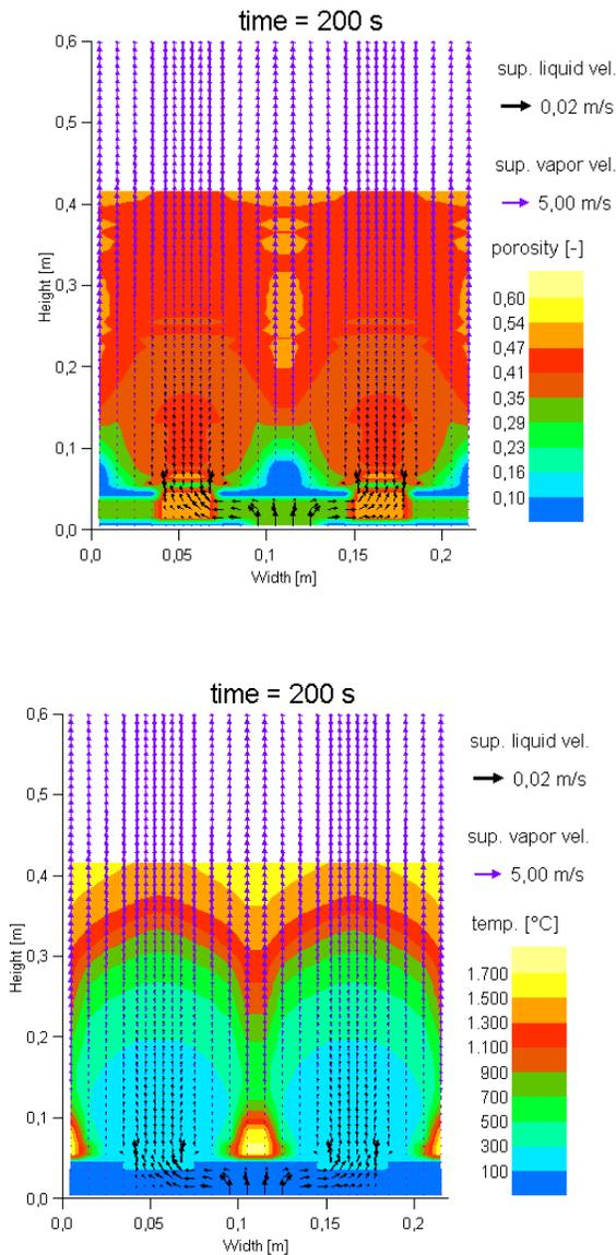
**Figure 12: VULCANO VW-U1 test of the COMET concept – WABE 2D Calculations**
