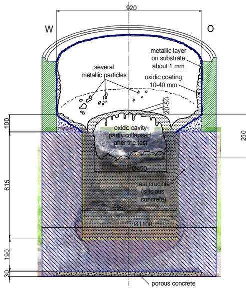
Figure 10: Final shape of the COMET L2 cavity
