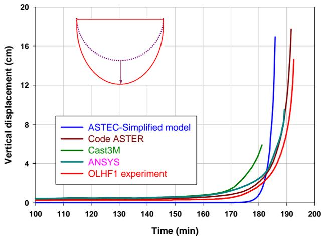
Figure 7: Comparison of OLHF-1 Calculations of the vessel displacement.
