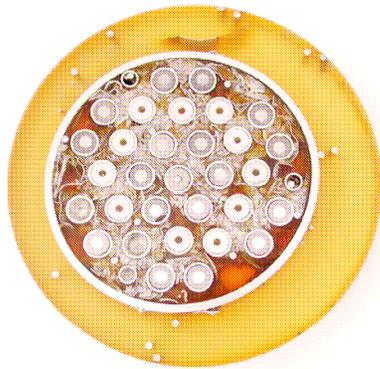
**Figure 1: The QUENCH-12 experiment. Observations of intense oxide scale spalling**
