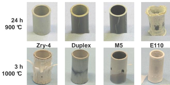
**Figure 2: Appearance of cladding materials after oxydation in Ar-O<sub>2</sub> atmospheres**
