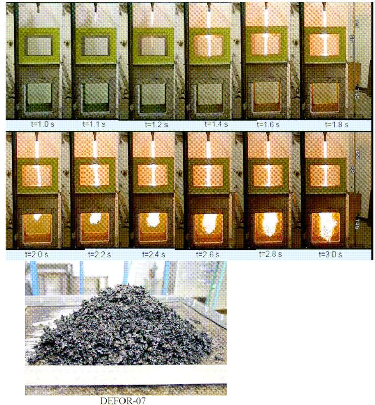
Figure 8: Sequence of melt pouring in water during a DEFOR test and typical debris bed.
