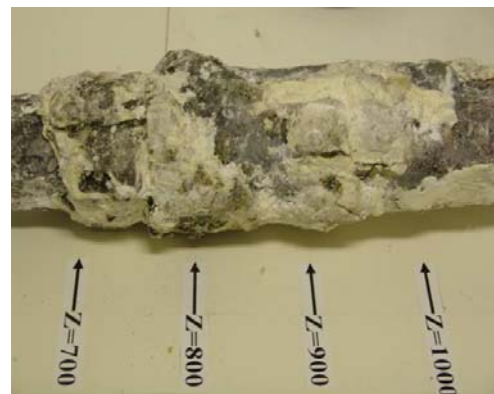
Fig. 8. Post-test appearance of the shroud (elevations of 700 – 1000 mm).
