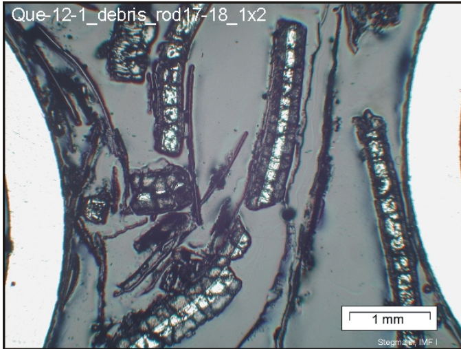
Debris fragments between two rods
