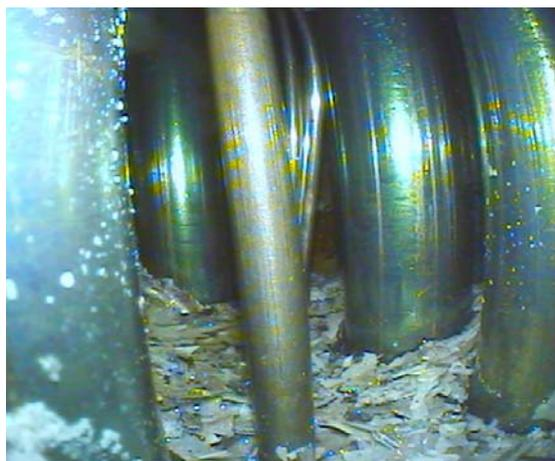
**Figure 3.** Spalled oxide scales, originated from rod claddings and shroud, were found after the test as debris at the bottom of the QUENCH-12 test bundle.
