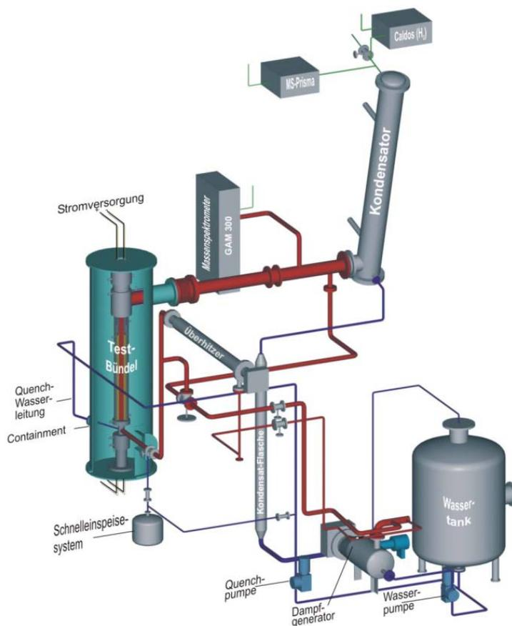
**Figure 1.** QUENCH test facility. Main emphasis is on the materials behavior at high temperatures and determination of the hydrogen source term during flooding of an overheated reactor core.
