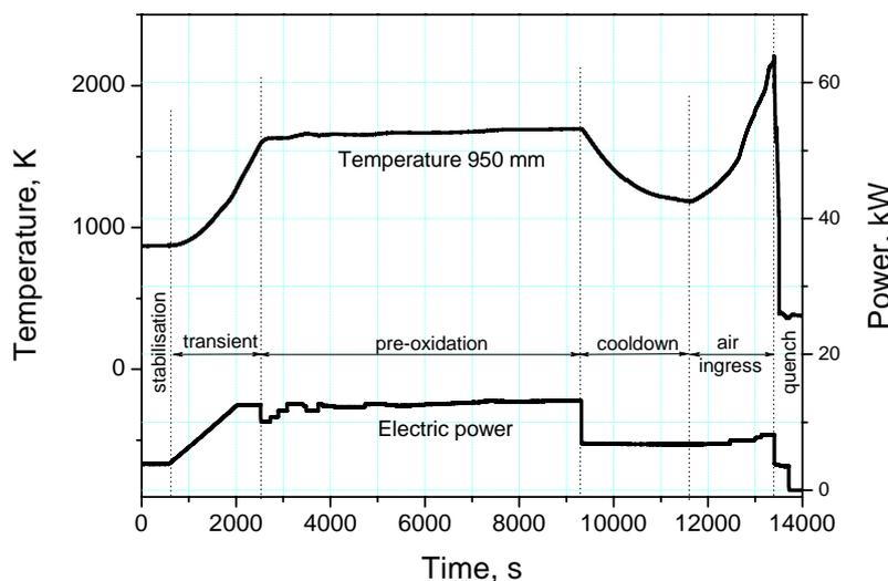
**Figure 2.** Temperature at the 950 mm level (TIT A/13) and electric power vs. time together with an indication of the QUENCH-10 test phases.
