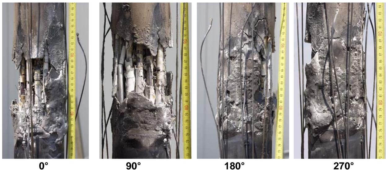
**Figure 4.** Posttest appearance of the QUENCH-10 bundle between elevations 730 and 950 mm at four different orientations. A portion of bundle and shroud broke off during dismantling due to extreme brittleness caused by Zr oxidation.
