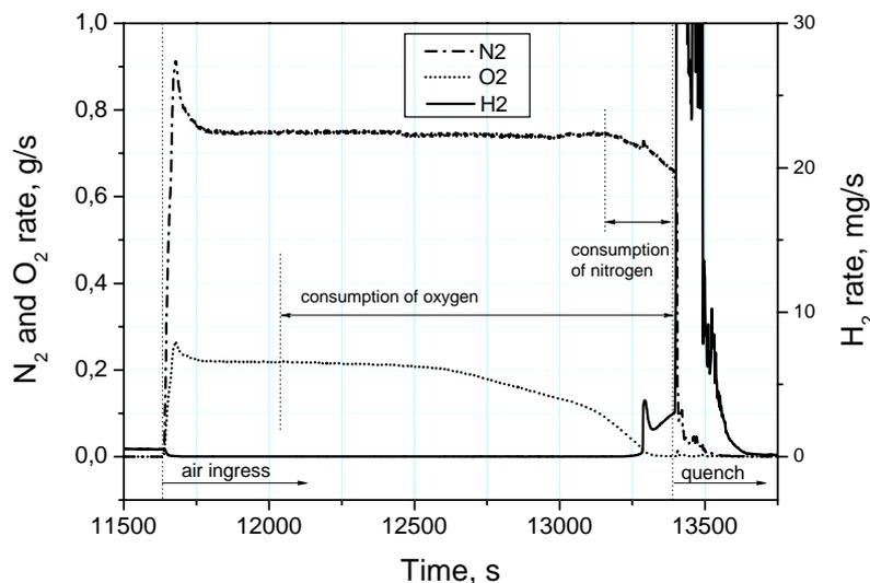
**Figure 3.** Mass spectrometer measurements of  $\text{H}_2$ ,  $\text{N}_2$ , and  $\text{O}_2$  during the air ingress phase of QUENCH-10. A small amount of hydrogen (note: scale is mg/s!) is released when oxygen is almost completely consumed.
