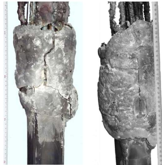
Fig. 6. Posttest appearance of the upper shroud regions of test bundles QUENCH-07 (left) and QUENCH-09 (right). The regions of shroud deformation are at elevations from  $\sim 810$  to  $1020$  and from  $\sim 560$  to  $>1000$  mm, respectively. The destruction inside the test bundle (which cannot be seen in these views) is more severe in QUENCH-09.
