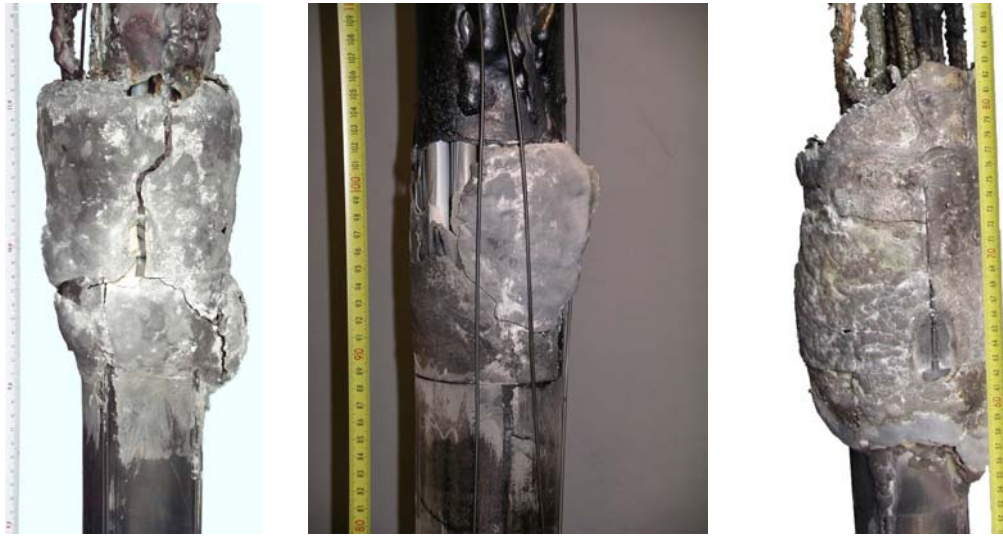
Figure 4: Posttest appearance of the shroud at the hot region (from ~750 mm upward) of test bundles QUENCH-07, QUENCH-08, and QUENCH-09 (from left).
