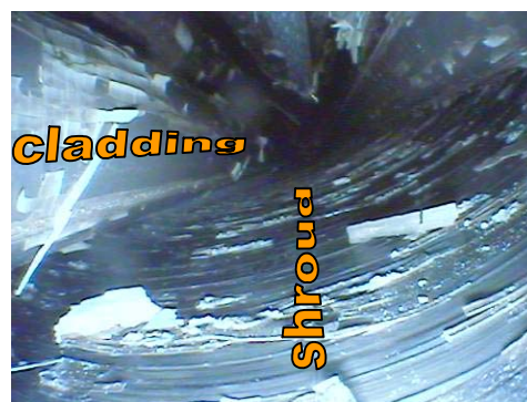
Fig. 15: QUENCH-12, videoscope inspection of breakaway effect at the 650 mm elevation. Cladding: E110, shroud: E125 alloy
