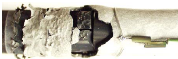
Figure 7: Fuel rod simulator specimen after pre-oxidation in steam, nitrogen reaction at 1300 °C and quenching in cold steam
