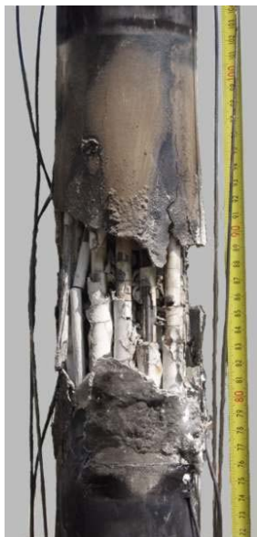
Figure 2: Post-test appearance of the QUENCH-10 bundle
