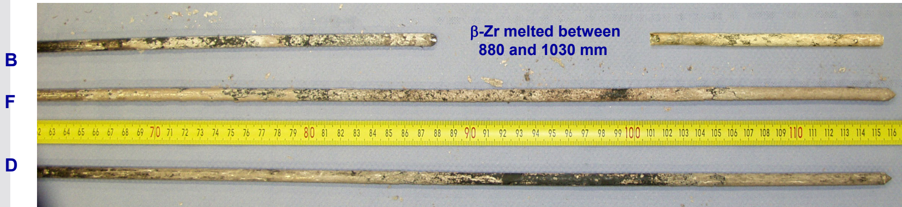
corner rods withdrawn during the test: spalling of the outer skin of oxide layer due to breakaway oxidation .
