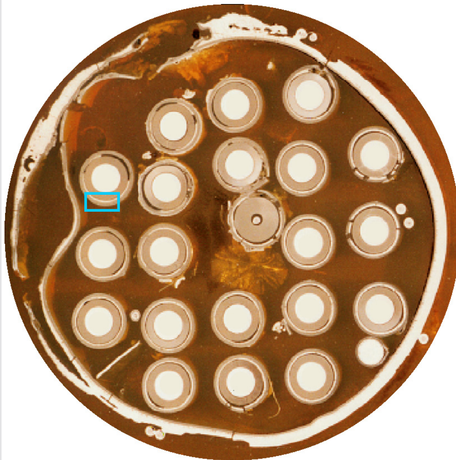
Q06 - bundle geometry intact-> good coolability; melt localized between pellet and ZrO 2 layer
