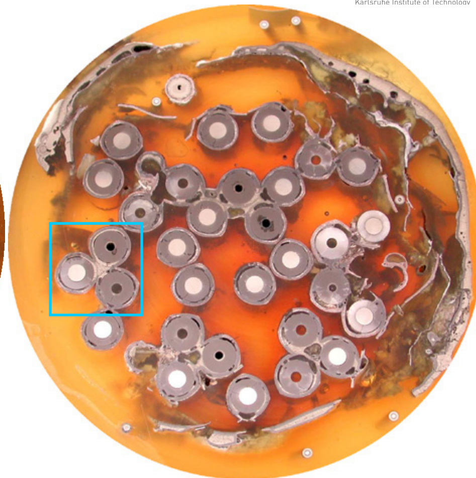
Q12 - bundle geometry destroyed-> declined coolability; molten pools formation inside rod clusters
