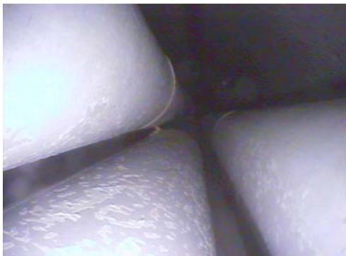
Fig. 10. Spalling of thin oxide scales at bundle elevation of 930 mm.
