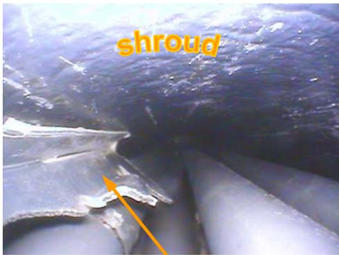
Fig. 9. Parts of destroyed grid spacer 4 at bundle elevation of 1030 mm
