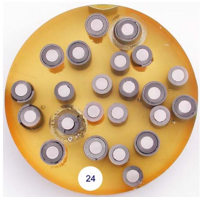
Fig. 12. Cross section of the QUENCH-15 bundle at elevation of 950 mm.
