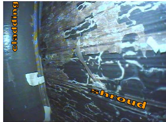
Fig. 9. Videoscope photograph with a side-view lens at elevation of 0.70 m: intensive oxide scale spalling on the coarse shroud surface.
