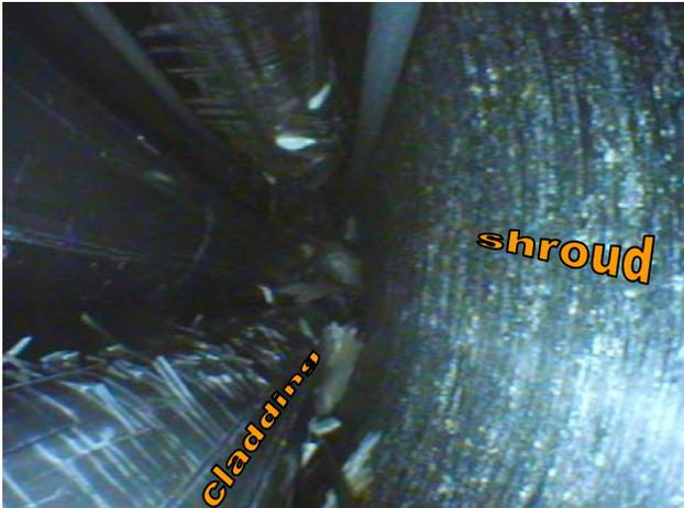
Fig. 7. Videoscope observation at bundle elevation 0.40 m at the empty position of corner rod F: circumferential spalling of the oxide layer on the surface of fuel rod simulator cladding.
