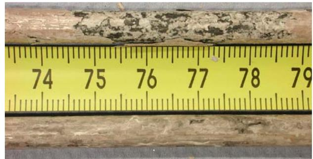
Fig. 4. The withdrawn corner rods D (lower) and F (upper) revealed breakaway oxidation with intensive spalling of oxide scales.
