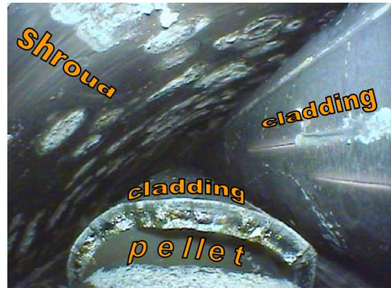
Fig. 10. Videoscope photograph at elevation of 0.90 m: circumferential and longitudinal cracks at the cladding; nodular breakaway corrosion at the shroud.
