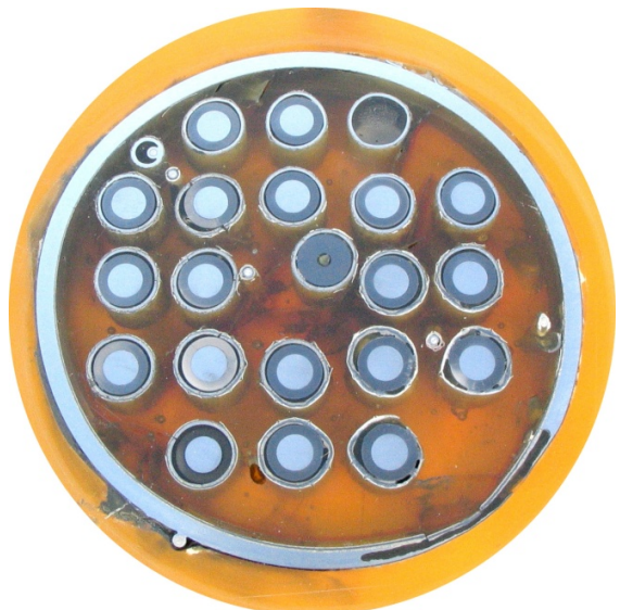
Fig. 9. Bundle cross section at 830 mm: minor melting of some cladding segments.
