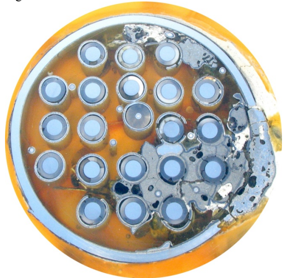
Fig. 8. Bundle cross section at 430 mm: frozen melt relocated from upper elevations.
