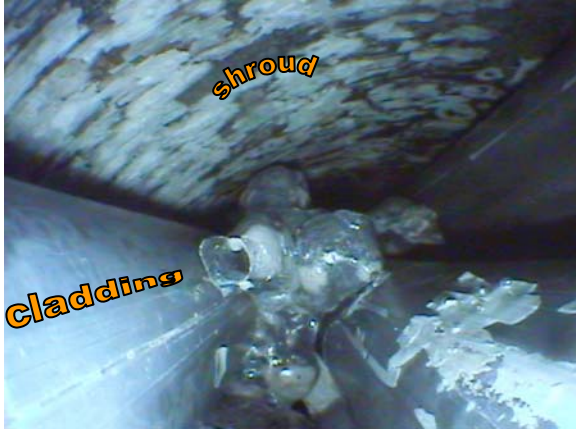
Fig. 8. Videoscope photograph at bundle elevation of 0.88 m: solidified melt of \beta -Zr part of corner rod B.
