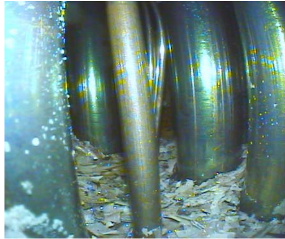
Fig. 14. Spalled oxide scales as debris at the bundle bottom.
