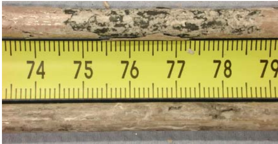
Fig. 4. The withdrawn corner rods D (lower) and F (upper) revealed a breakaway oxidation with intensive spalling of oxide scales.
