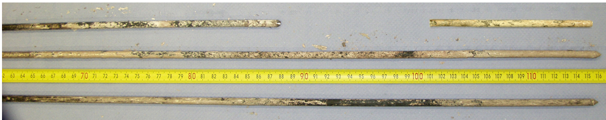
Figure 2. The withdrawn corner rods D (lower), F (middle), B (upper) revealed an extensive breakaway effect and spallation of oxide scales.
