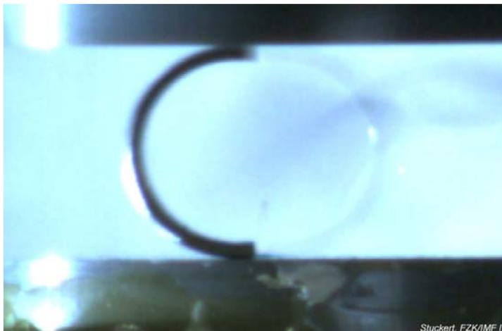
73.527 s: beginning of probe disintegration
