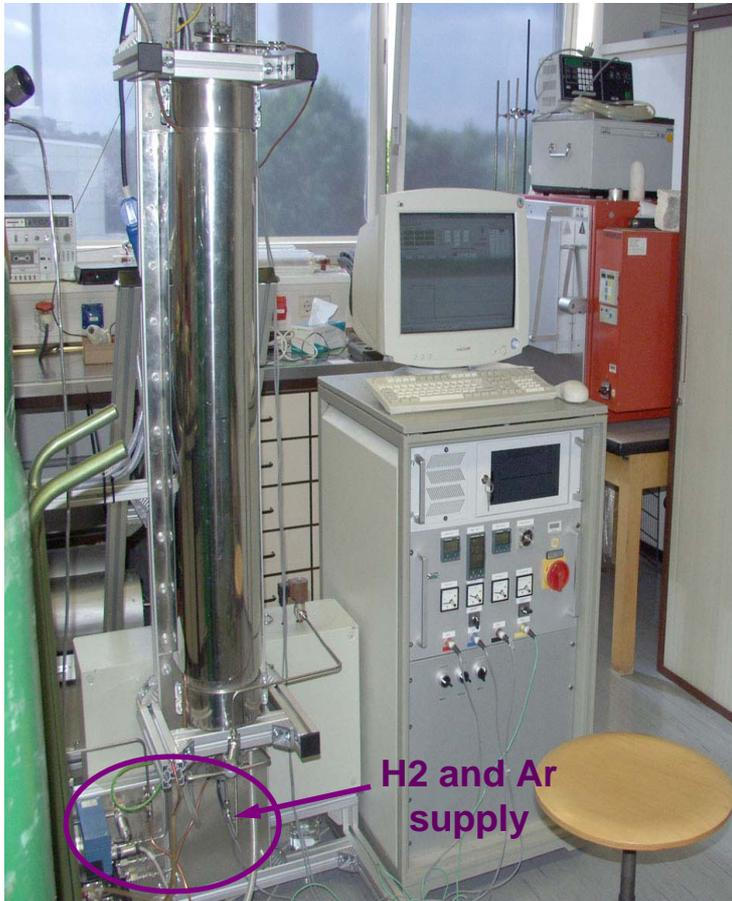
**vertical 3-zones tube furnace LORA
