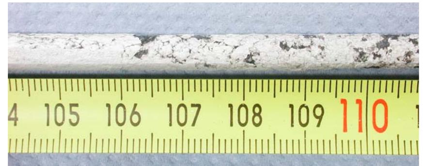
**corner rod E, E110: breakaway, intensive spalling of spongy oxide scales**
