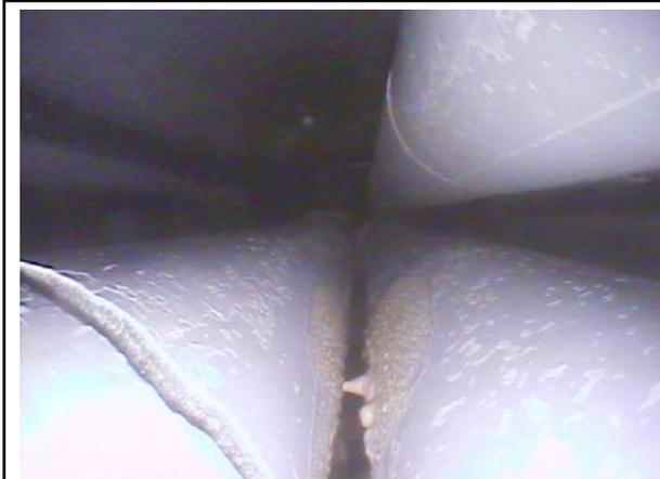
950 mm, circumferential cracks and negligible oxide spalling;
