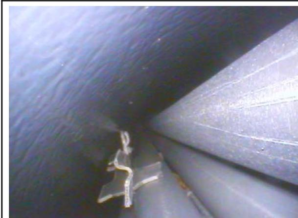
700 mm, relocated part of grid spacer 4
