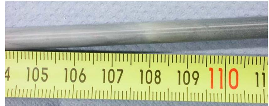
**corner rod D, Zry-4: no breakaway, no oxide spalling**
