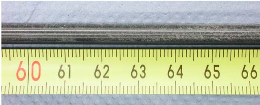
**corner rod A, Zry-4: negligible breakaway, no oxide spalling**
