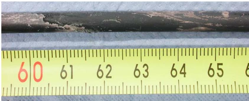
**corner rod E, E110: breakaway, intensive spalling of oxide scales**
