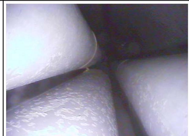
930 mm, spalling of thin oxide scales
