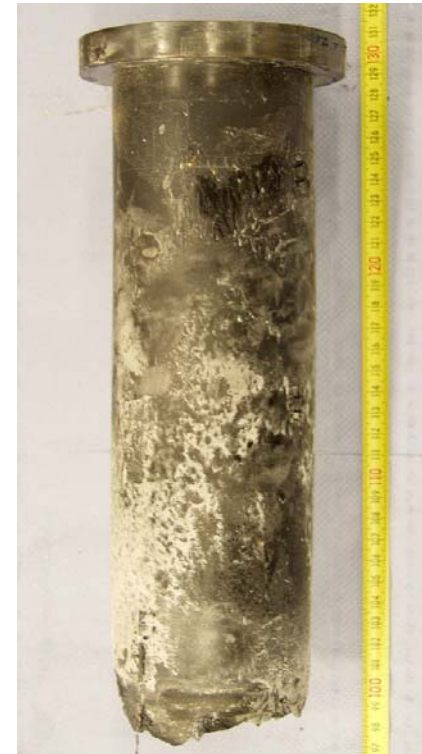
upper part of the shroud braked off from the bundle during dismantling (angle position of 180°)
