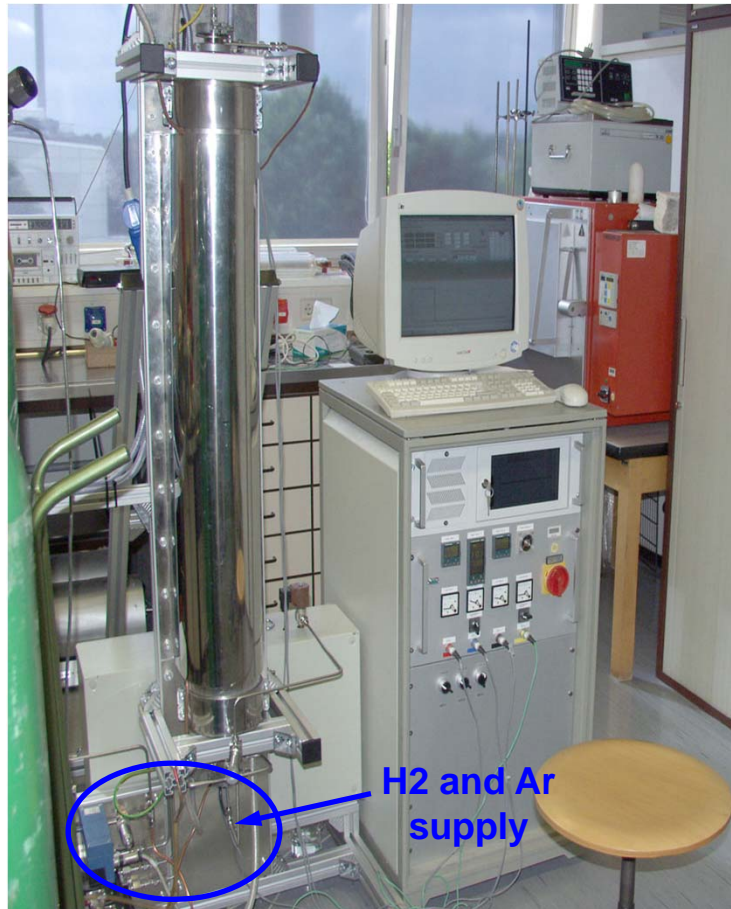
vertical 3-zones tube furnace LORA (height 60 cm)
