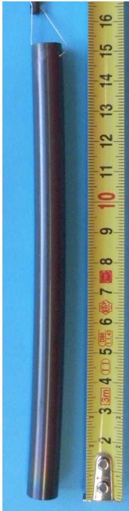
H14Z4: annealed at 700 °C with H 2 (37 mbar); \Delta t=240 s \Delta m_H=1800 wppm
