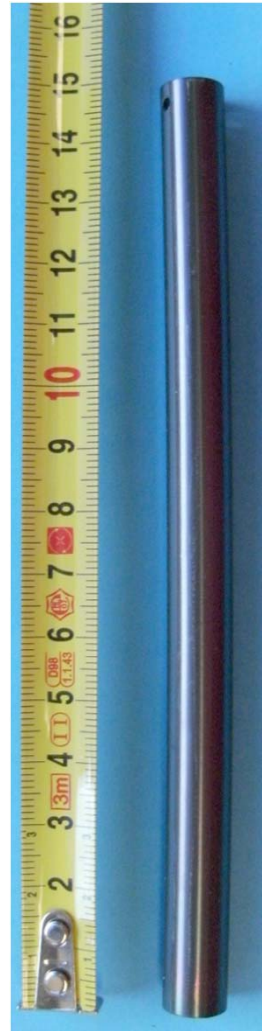
H19Z4: annealed at 800 °C with H 2 (37 mbar); \Delta t=240 s \Delta m_H=1600 wppm
