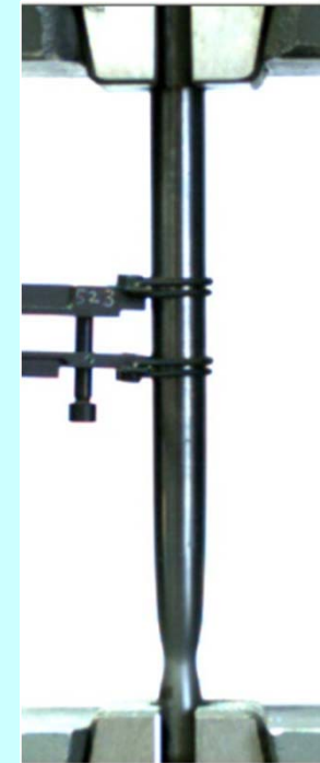
ductile not hydrogenated probe with pronounced contraction
