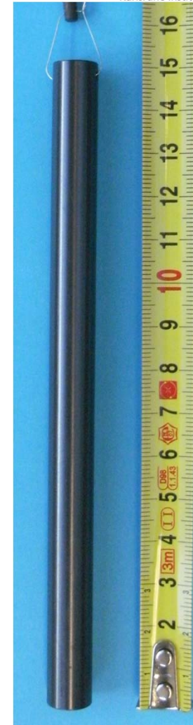
H33Z4: annealed at 900 °C with H 2 (37 mbar); \Delta t=480 s \Delta m_H=1700 wppm
