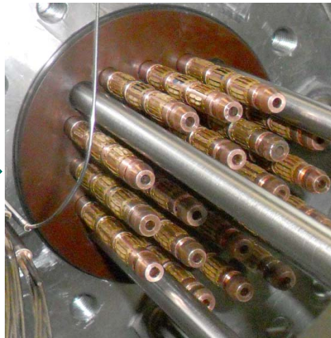
Cu electrodes with Au slide contacts
