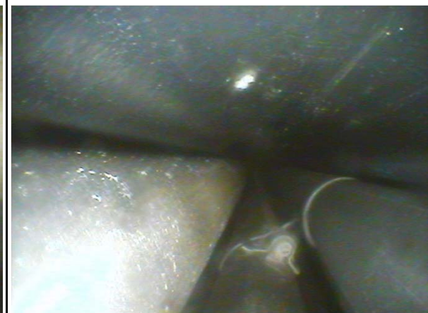
1150 mm: intact dark oxidised surface of claddings
