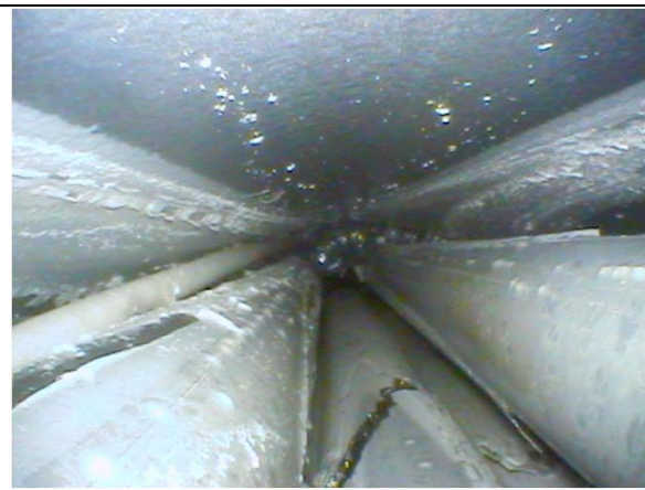
350 mm: oxide cracks; between rods – melt relocated from upper elevations
