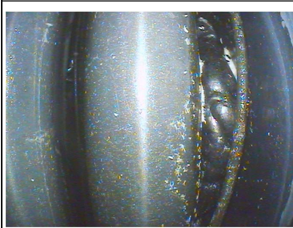
215 mm: frozen melt relocated from upper elevations
