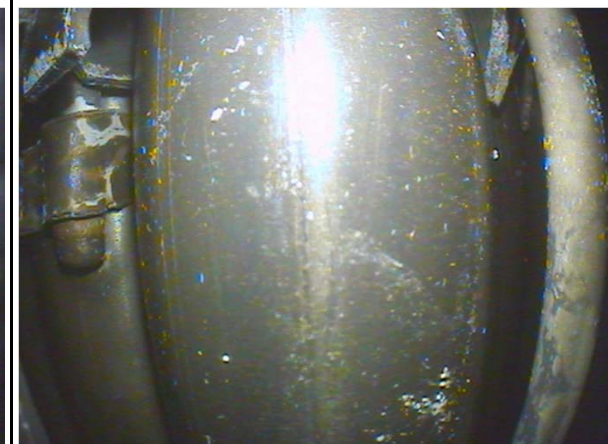
1050 mm: dark oxide of claddings, intact Grid Spacer #4
