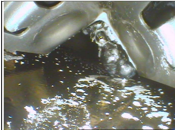
Grid spacer #1 at -60 mm: frozen melt relocated from upper elevations
