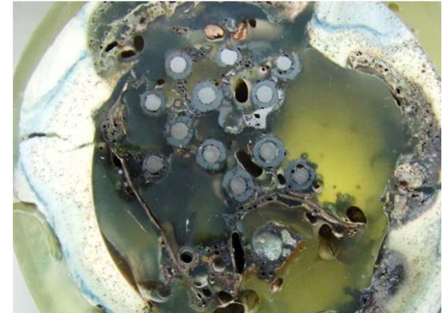
1200 mm: melt; nitrides dissolved by melt
