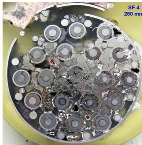
260 mm: rods partially dissolved by relocated melt
