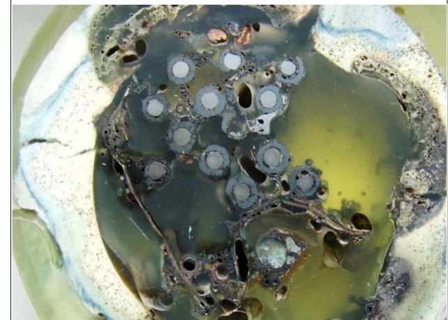
1200 mm: absence of melted claddings
