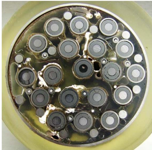
130 mm: intact rods, small melt pools
