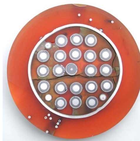
750 mm: oxidised claddings
