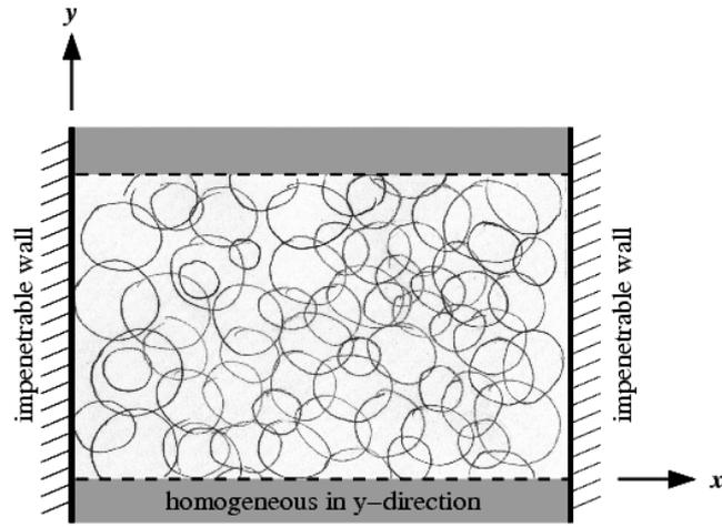
**Fig. 1:** Sketch of a distribution of dislocation loops in a constrained slip channel. We consider a one-dimensional special case where the movement of dislocations is hindered by impenetrable walls at the left and the right side of the geometry, while assuming an infinitely long and homogeneous distribution in  $y$ -direction. Close to the walls line orientations parallel to the walls dominate the distribution
