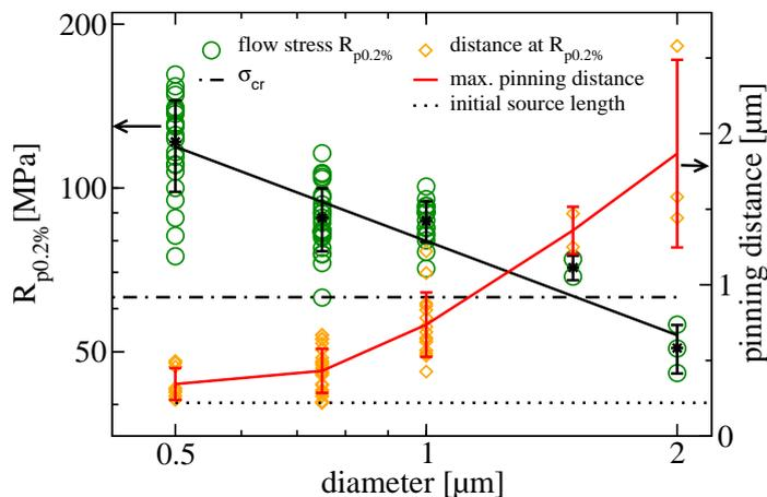
**Fig. 1:** Flow stresses at 0.2% plastic deformation to the left and dislocation length, characteristic for the weakest structure to the right (Scripta Mater. 2008; Mat Sci Eng A. 2008)
