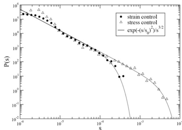
**Fig. 2:** Strain burst distribution for stress and strain control;  $s$  is a measure for the strain burst size and  $P(s)$  is the probability of occurrence
