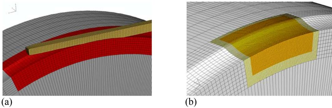
**Fig. 2:** (a) Wire rolling 3-D FE mesh, (b) element set provided FE data to run reliability analysis in STAU
