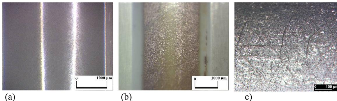
**Fig. 3:** (a) Caliber surface before running the experiments, (b) copper adhesion on the caliber surface, (c) surface cracks on the caliber
