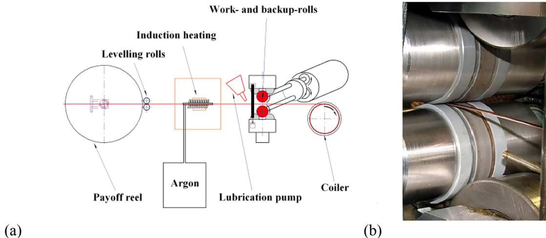
**Fig. 1:** (a) Wire rolling test rig, (b) work rolls are arranged in a cluster mill configuration
