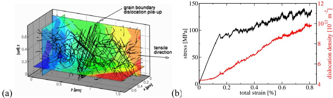
**Fig. 1:** (a) Pillar with a horizontal GB (arrow) under tensile loading. Dislocations (black lines) and displacement in tensile direction due to dislocations at 0.8% total strain are presented. b) Stress strain curve and evolution of dislocation density of pillar
