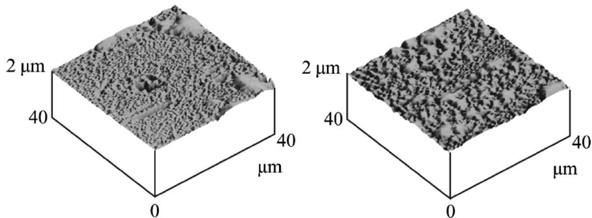
**Fig. 1:** Atomic force microscopy images of a grey cast iron sample after a friction experiment with 30 N (left hand side) and 90 N (right hand side) normal force. The different wavy topography features have emerged as a result of different sliding conditions. Adapted from [M. Scherge et. al., *Wear* 255, 395 (2003)]
