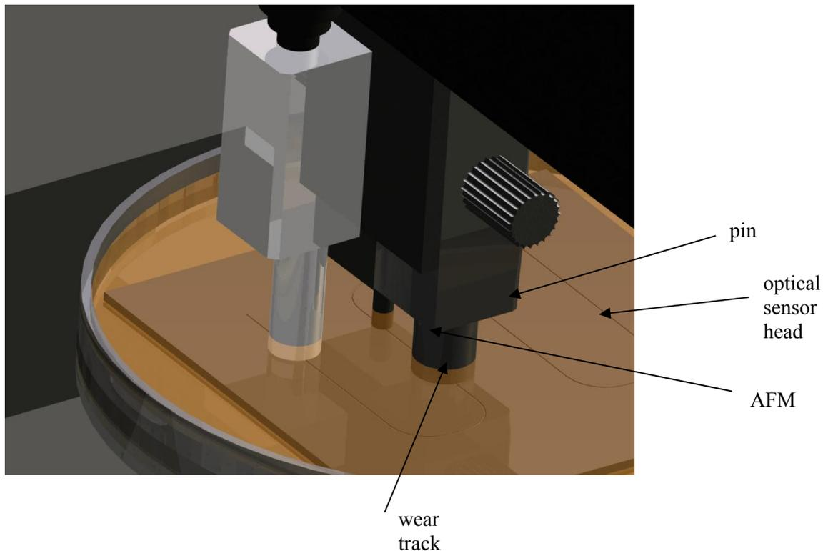
**Fig. 2:** CAD model of the experimental platform which is currently being set up, showing the sliding pin and an atomic force microscope (AFM) and an optical sensor
