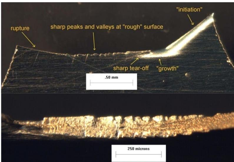
**Fig. 3:** Optical micrographs show the fracture surface of an nc-Ni fatigue sample
