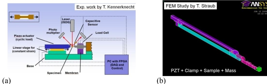
**Fig. 1:** a) The sketch shows the custom built micro-fatigue setup consisting of a linear stage, a piezostack, the sample and a load cell. Strain can be measured by the use of a laser interferometric technique as well as with a camera and digital image correlation and tracking. Fig. 1b shows the FEM model of the used piezostack (blue) in a steel casing (violet) and a sample attached to the sample grip (pink) with a small mass (green) at the end that is designed to work at 1kHz
