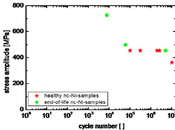
**Fig. 2:** Wöhler-diagram of nc-Ni samples. To be able to observe ongoing damage mechanism, the experiments were interrupted to conserve different states in the lifetime of these samples
