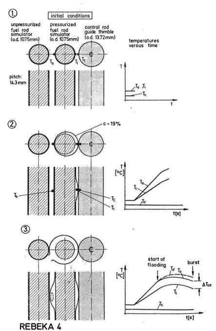
Cladding deformation mechanism under the influence of a cold control rod guide tube (schematic)
