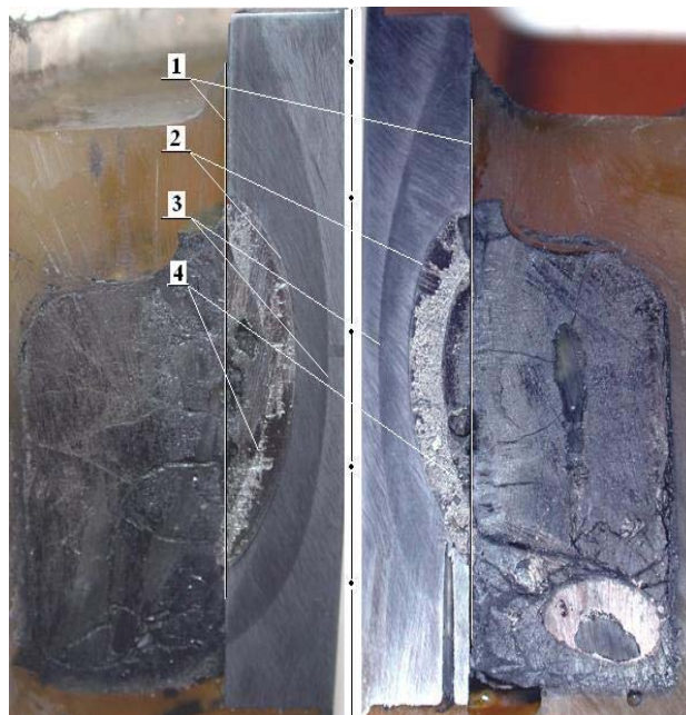
1 – conventional lateral surface of the initial steel specimen; 2 – corium/steel interaction zone boundary; 3 – boundary of the zone of molten corium thermal impact on steel structure; 4 – boundary between two parts of the interaction zone.
