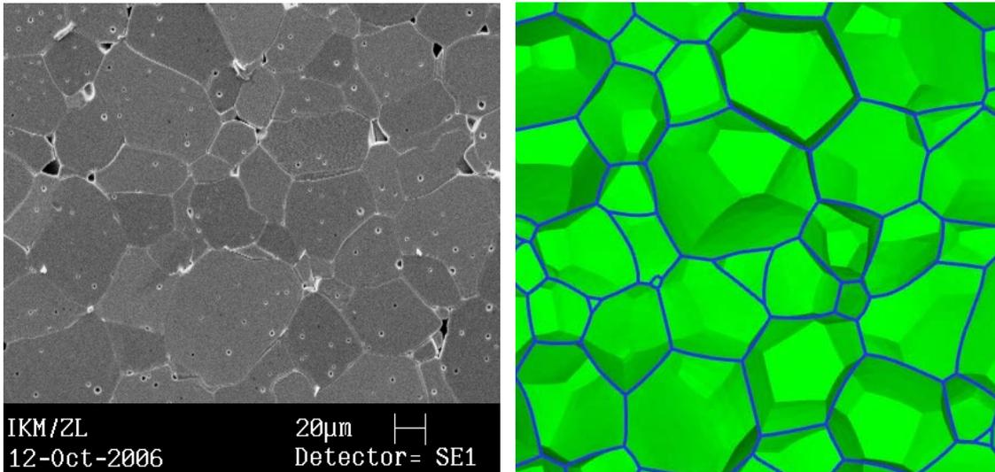
**Fig. 1:** 2D cross section from (a) experiment and (b) simulation
