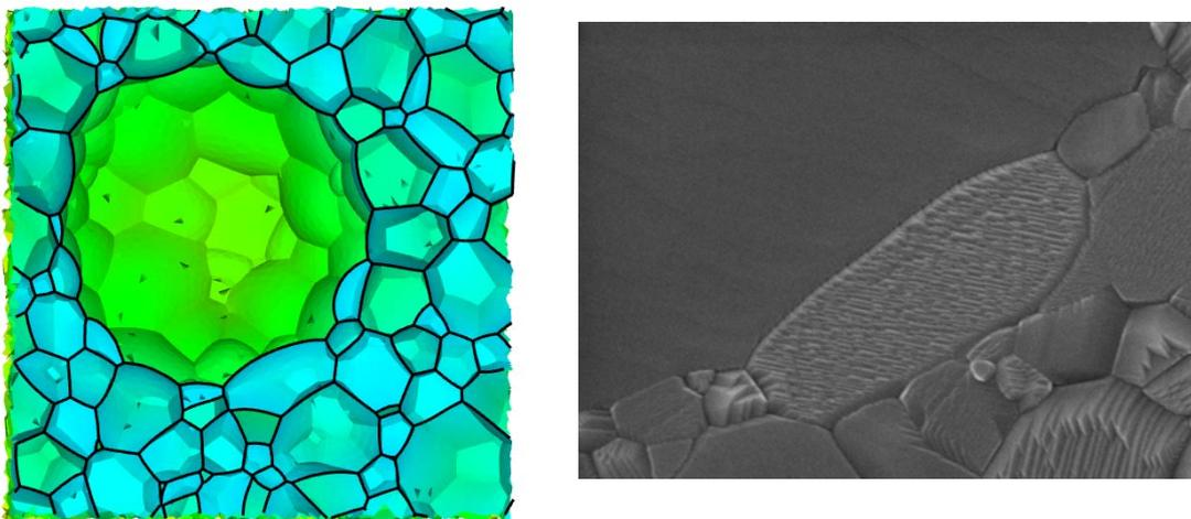
**Fig. 2:** Abnormal grain growth in simulation and experiments on STO Ceramics: (a) abnormal grain and matrix grains; (b) experiments performed at the IKM (M. Bäurer, M. Hoffmann)
