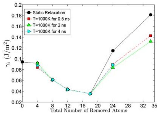
**Fig. 2:** Interface excess energy as a function of the number of vacancies at the interface
