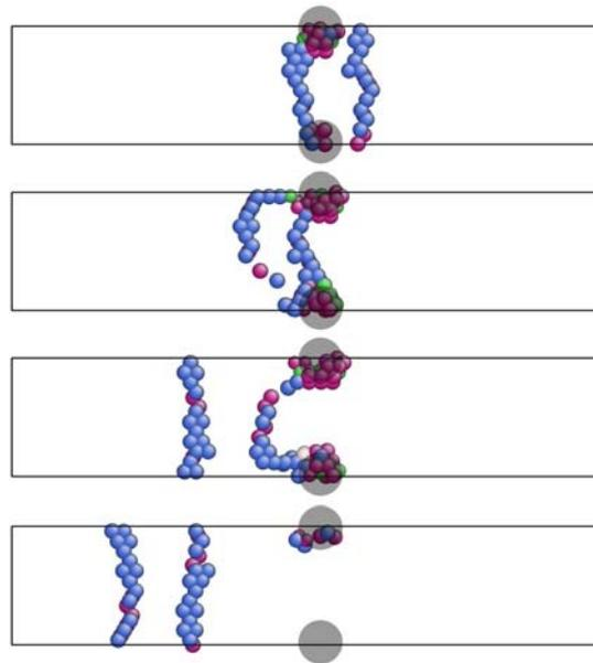
**Fig. 2:** Interaction of a moving dislocation in Al with a Cu- cluster (grey circle)
