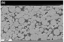
Cross-section of a battery electrode with porous nanostructured particles. [1]
