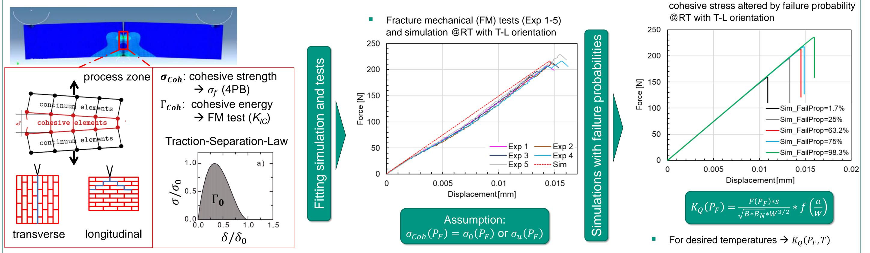
Step 1: Keep cohesive stress ( $\sigma_{Coh}(63.2 \%)$ ) constant and alter cohesive energy ( $\Gamma_{Coh}$ ) to fit simulation result to experimental result
