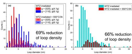
Dislocation loops size distributions for the as-irradiated (15 dpa, 330 °C) and PIA (550 °C/3 h) EUROFER97 samples estimated via (a) WBDF and (b) HAADF-STEM techniques
