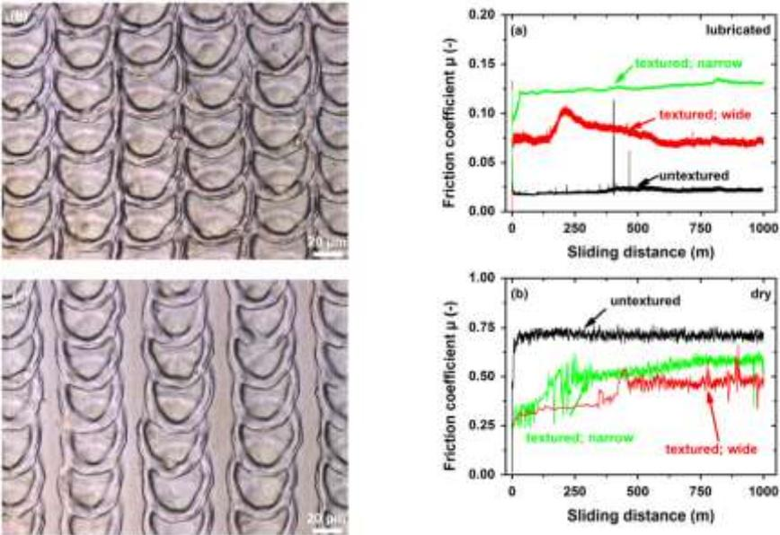
Images of bio-inspired surface morphologies created through laser surface texturing (left) and their effect on friction coefficient in lubricated and dry condition (right) from [2].
