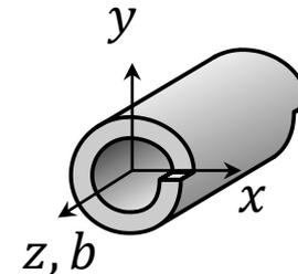
$$(\sigma_{ik}) = \begin{pmatrix} 0 & 0 & \tau_{xz} \\ 0 & 0 & \tau_{yz} \\ \tau_{xz} & \tau_{yz} & 0 \end{pmatrix} = \frac{G \cdot b}{2\pi} \begin{pmatrix} 0 & 0 & -\frac{y}{x^2 + y^2} \\ 0 & 0 & \frac{x}{x^2 + y^2} \\ -\frac{y}{x^2 + y^2} & \frac{x}{x^2 + y^2} & 0 \end{pmatrix}$$
