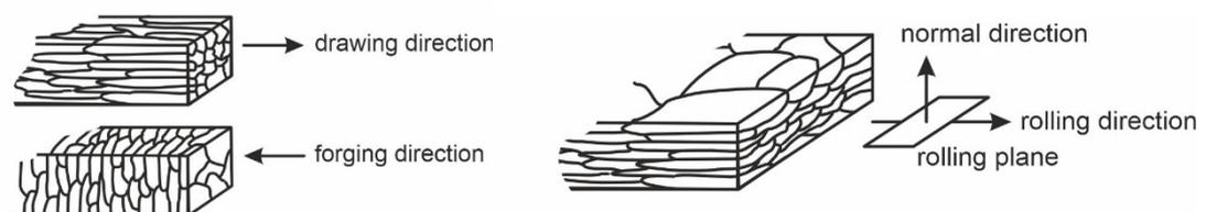
Figure 1: Schematic representation of different sections of wires and forged parts (left) and rolling (right) according to Ref. [1].
