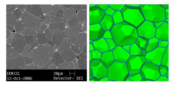
Fig. 1: 2D cross section from (a) experiment and (b) simulation
