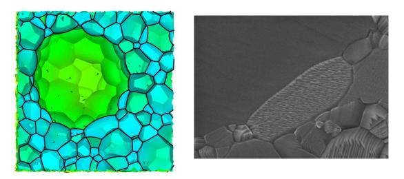
**Fig. 2**: Abnormal grain growth in simulation and experiments on STO Ceramics: (a) abnormal grain and matrix grains; (b) experiments performed at the IKM (M. Bäurer, M. Hoffmann)
