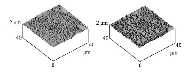
**Fig. 1**: Atomic force microscopy images of a grey cast iron sample after a friction experiment with 30 N (left hand side) and 90 N (right hand side) normal force. The different wavy topography features have emerged as a result of different sliding conditions. Adapted from [M. Scherge et. al., Wear 255, 395 (2003)]
